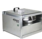
CL/PLUS/EC In-line extract fans for rectangular ducts with a 40 mm thick acoustic casing to reduce noise and EC Technology motor
